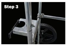
Place your post driver on to the cart cradle and make sure the height is correct for your post driver and that all hardware is tightened.
