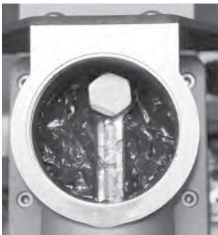
Fig. 11 - After completely cleaning out old lubricant, add new Rhino® Pro Series Lubricant till level with the bottom edge of the crank pin head.
