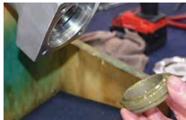
Fig. 16.2 - Insert the Anvil O-ring Retainer with correct radius facing UP
