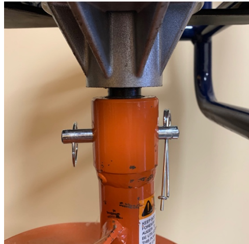
Positioning an auger (Fig. 1)
