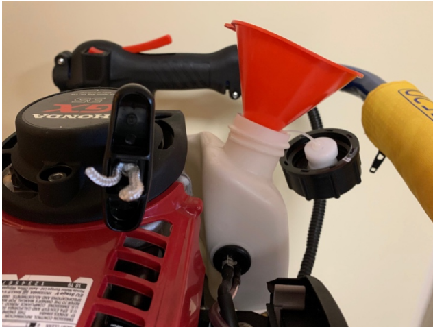
Figure 3 – Filling the tank with fuel
